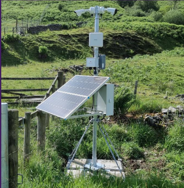
Left: solar-powered people counting cameras and air quality sensor at Destination Tweed Right: air quality sensor at Stranraer Harbour Office
